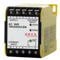
Final calibration is trimmed using the front accessible 'offs' and 'span' 15-turn trim adjustments. Various power supply choices are available ranging from 415Vac down to 12Vdc. These transducers are Australian designed and manufactured and offer a vast range of input to output combinations.
