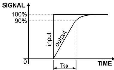
T90 is defined as: for an input step of 0 - 100%, the output ramps up to 90% in T90 seconds, i.e. 18.4mA for 4 - 20mA input.
