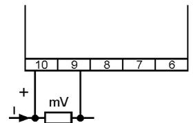
Input range bipolar:  $\pm 0.5\text{mV}$  to  $\pm 2\text{kV}$
