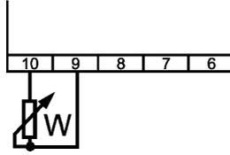
Input span: 2Ω up to 5kΩ (reverse action on request)
