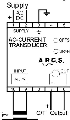
The example shown uses an external current transformer; in many cases this is not necessary as the ACT141 can directly accept up to 10A.
