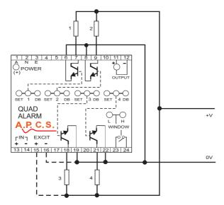
This drawing shows all emitters commoned and external pull-up resistors to an external power supply.
