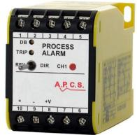
The standard version has one change-over contact, 240V rated. A second change-over contact rated up to 48Vdc can be wired to terminals 6, 7 and 8 as an option. Dead band is continuously adjustable from 0.5 to 10% of range via 15-turn trimmer on front (DB). A 0.5 second filter for fluctuating process signals is standard with all units, but can be decreased or eliminated where fast response is important.
