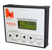
The "**Trim Mode**" is used to change selected parameters for each previously programmed input, output and equation constant to an operating USC701 without disruption to output function. The "Trim Mode" can be used in conjunction with the "USC Config" program to create a customised user interface for each USC701.
